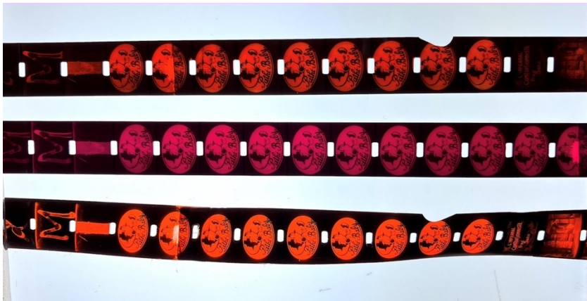
Fig. 11: Reconstructions of the Barzizza 9.5mm film print in orange-red colour and with notch on the edge. With the original Barzizza film at the bottom, the first copy in the middle, and the last copy with only red food colouring on top.
